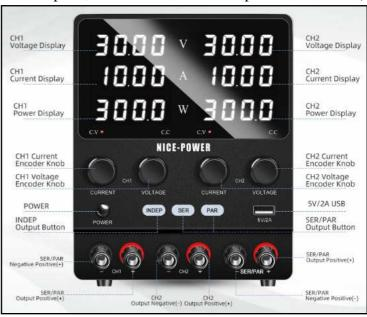
in this case max. 240 V can be measured. If the + poles and the - poles are connected, the max. 120 V, but the load capacity doubles, it will be 6 A (720W). An interesting feature of this power supply is
